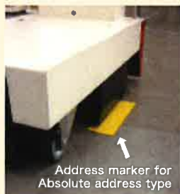
※We provide buried type magnetic cable and spot marker. ※Can be coated magnetic tape and spot marker with plastic.
